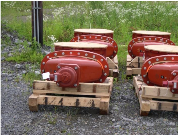
Large Gate Valves.
